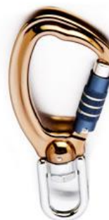
Alu trilock karabiner acc. to EN 362 mounted on strap fall arrester 25 KN Opening width 22 mm
